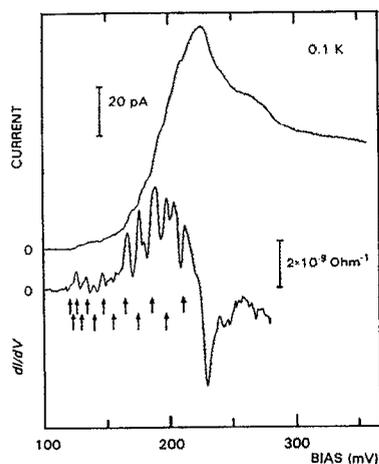
FIG. 3.  $I$ - $V$  and  $dI/dV$  vs  $V$  curves (positive bias) for the  $D = 0.6 \mu\text{m}$  device. The arrows give the positions of the peaks in  $dI/dV$  vs  $V$  calculated from the model described in the text. The upper row are the  $m = 0$  states and the lower row are the  $m = 1$  states. From left to right,  $n = 1, 2, 3, \dots$
