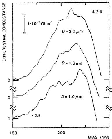
FIG. 2.  $dI/dV$  vs  $V$  curves (positive bias only) for three different size devices, where  $D$  is the Au-Ni-Ge contact (etching mask) diameter. The structure in the differential resistance is due to lateral size quantization.
