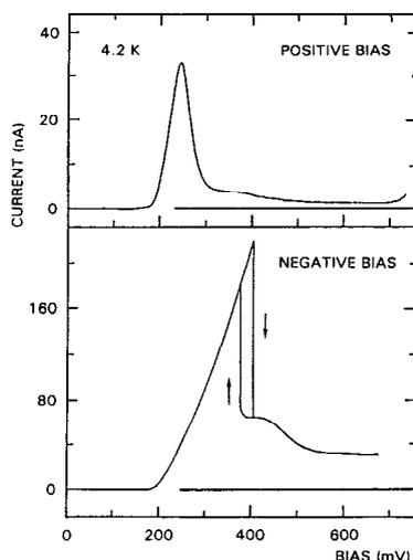
FIG. 1.  $I$ - $V$  curve of a large-area device ( $D = 2.8 \mu\text{m}$ ) at 4.2 K. The asymmetry of the  $I$ - $V$  curve for positive/negative bias is due to the asymmetry in the barrier material composition (height).
