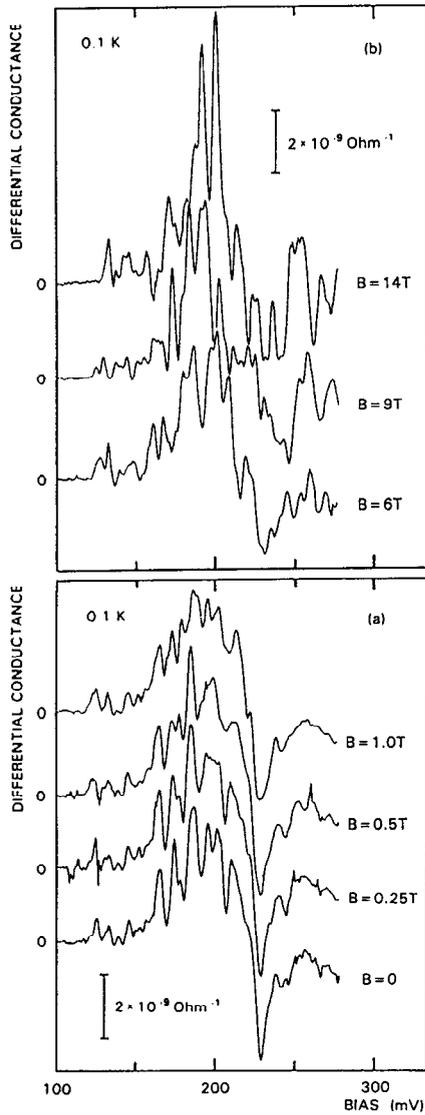
FIG. 4.  $dI/dV$  vs  $V$  curves for the  $D = 0.6 \mu\text{m}$  device of Fig. 3 in a magnetic field parallel to the tunneling direction.
