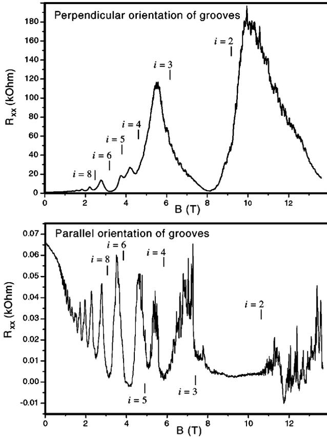
FIG. 4. The longitudinal resistance  $R_{xx}$  versus magnetic field for both sample orientations,  $T=20$  mK. The vertical dashes give positions in  $B$  of corresponding  $R_{xy}$  plateaus or maxima in Fig. 3.
