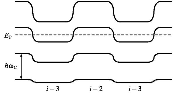
FIG. 5. A schematic diagram of Landau levels for a V-grooved sample. The filling factor is less for the flat regions at the top and bottom of a V groove perpendicular to  $B$ , and greater at the sidewalls, inclined to  $B$  at approximately  $49^\circ$ . Spin splitting is neglected here.
