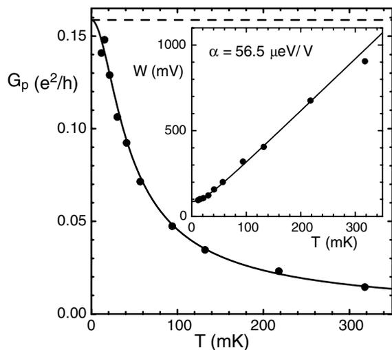
FIG. 5. Peak tunneling conductance  $G_p$  vs temperature  $T$ . For  $35 < T < 320$  mK,  $G_p \propto 1/T$  (solid line), as expected for resonant tunneling through only one nondegenerate state. The dashed line gives the expectation for tunneling through a ring of degenerate states, with Coulomb blockade lifting degeneracy. Inset shows the dependence of the width parameter  $W$ ; for  $T > 35$  mK,  $W \propto T$  (solid line).
