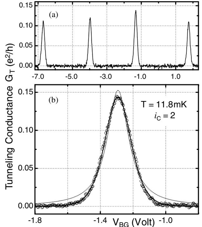
FIG. 4. (a)  $G_T$  vs  $V_{BG}$  for  $R_{xx}$  dips on the low- $B$  side of the  $i_C = 2$  plateau at  $B = 0.804$  T. (b) High-resolution sweep data (circles) of one of the peaks. Solid line is the best fit to Eq. (4). Dotted line is the best fit to a Lorentzian Eq. (5).
